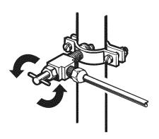
**ACAUTION:** Check to see if leaks occur at the water line connections.
